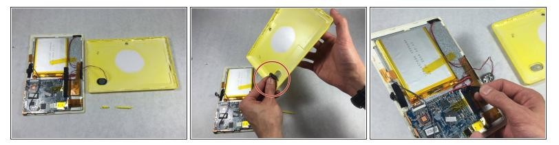
Once the casing is off, carefully pull the speaker out of its plastic holding slot, be careful not to separate the connections to the wires.
