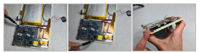
Next, remove the 4 screws that hold the mother board in place. Allowing the motherboard to wiggle in place.
