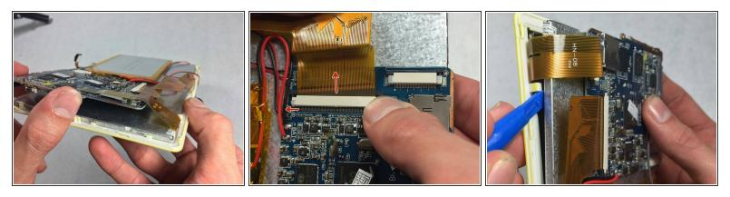
• Now that the motherboard is disconnected, disconnect the longer flat cables by pushing the locks open and taking the cable out.
