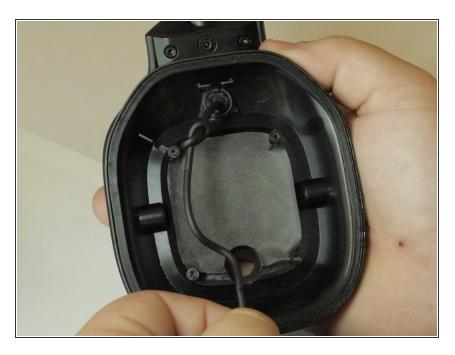
Untile the disconnected wiring harness.
