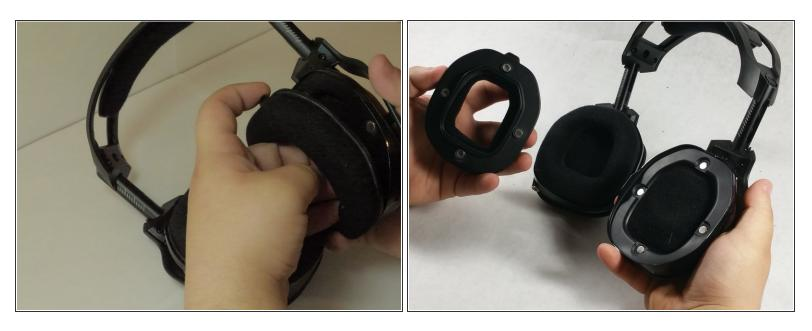
• To access the speakers you need to disassemble the earpiece. First remove the foam ear piece by simply pinching the padding and pulling lightly until the magnets disengage.
