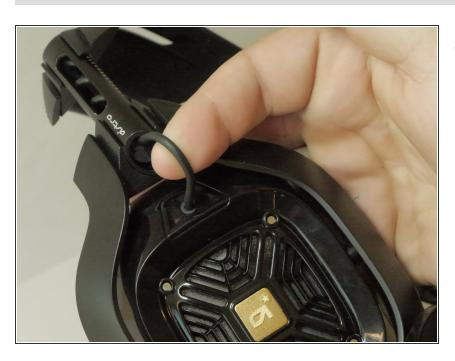
Pull the black wire out of the hole in the device.
