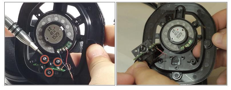
Locate the three small screws under the speaker. Use the J00 Philips Driver to remove them.
