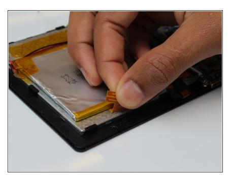
Remove the orange tab from the back of the screen as shown in the picture
