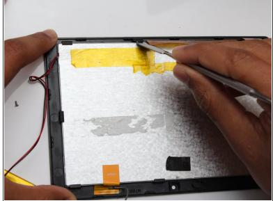
• Use the flat end of the metal spudger to unclip and remove the screen from the casing.
