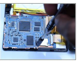
Using a Phillips screwdriver (PH00), unscrew the motherboard from the device
