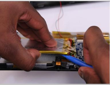
Use the flat end of the spudger to gently pry the battery from the back of the screen.
