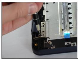
Unscrew the four screws using Philips #2 screwdriver that connect the screen to the inside of the case for the laptop.
