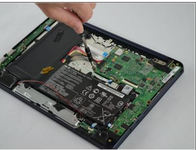
Unscrew all seven screws around the outer edge of the motherboard using 2mm Phillips Screwdriver.
