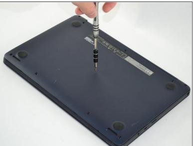
Unscrew all 10 2mm screws located on the bottom of the laptop using a Phillips #2 screwdriver.
