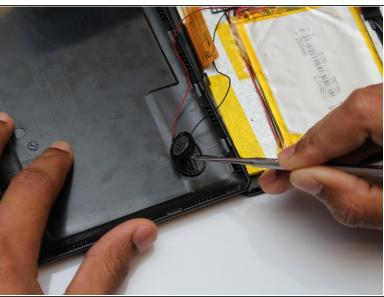
Using a spudger gently remove the speaker from the back of the device.
