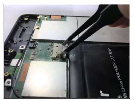
• Use tweezers to carefully disconnect the power cable bundle from the motherboard.
