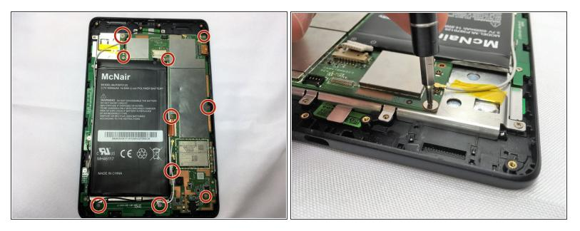
Remove the 10 screws from the motherboard using a Phillips #0 screwdriver.
