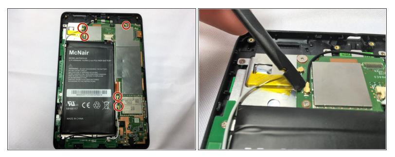
• Using a spudger, remove the 5 antenna cable connectors from the motherboard.
