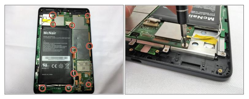
Use a Phillips #0 screwdriver to remove the 10 screws from the motherboard.
