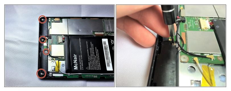
Remove 2 screws from each speaker, 4 screws in total, using a Phillips #00 screwdriver.
