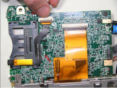
Peel back the tape on the camera ribbon cable connector.
