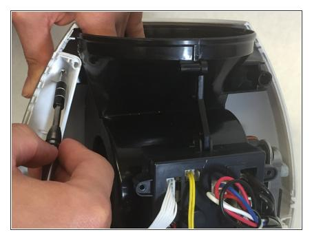
Locate the screw that was being hidden by the control board and remove it to release the second half of the shell.
