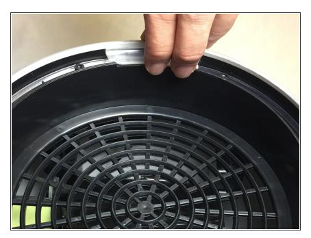
Using two fingers lift the translucent LED cover from the inside. Repeat this step for the second tab.
