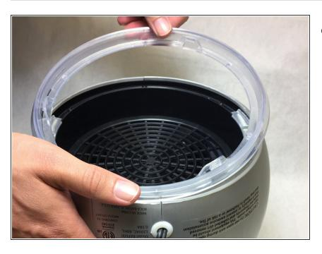
After the 6 screws are removed, remove the LED housing from the bottom of the device by lifting it off.
