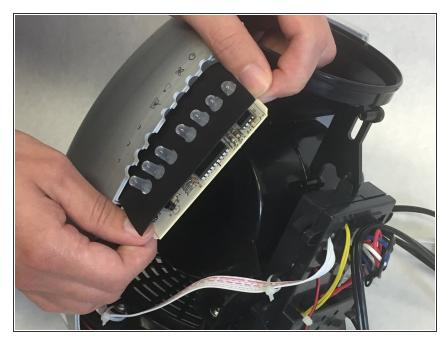
Locate the control board and grab it by the top and bottom firmly. Pull the board straight out being careful not to flex the circuit while removing.
