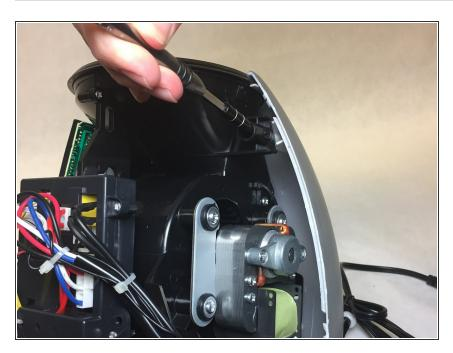
Locate the screw housing opposite of the control board, and remove the screw.
