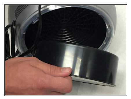
Grab the edge of the filter housing and pull the filter away from the rest of the device.
