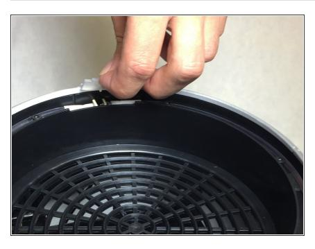
After lifting 45 degrees, pull the translucent tab away from thee housing. Repeat this step for the second LED cover.
