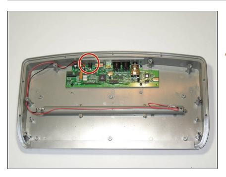
The power plug port in soldered onto the motherboard, and screwed onto the back plate.
