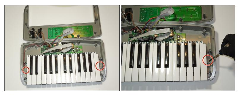
Remove the two highlighted 10 mm M3 galvanized machine screws using the J1 head fro the iFixit Tool Kit or a comparable tool.
