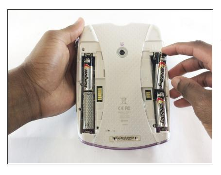
Remove the AA batteries from both battery compartments of the device.
