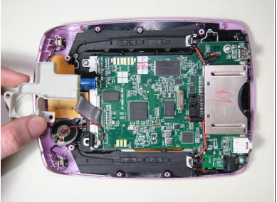
Remove the plastic speaker holder from the device.
