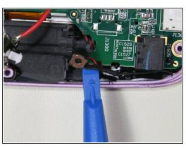
Use the small plastic opening tool to gently lift under the side microphone's black wire to remove the microphone from its slot.
