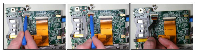
Open the camera connector by lifting on the brown latch with a plastic opening tool or a finger until it is in a vertical position.
