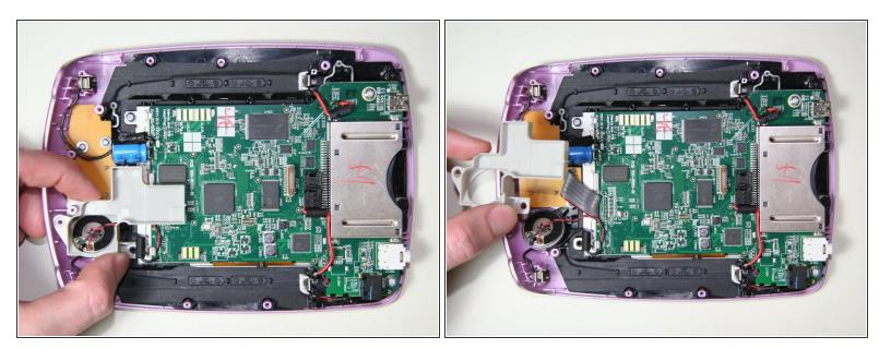
• Remove the plastic speaker holder from the device.
