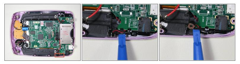
Use the small plastic opening tool to gently lift under the side microphone's black wire to remove the microphone from its slot.
