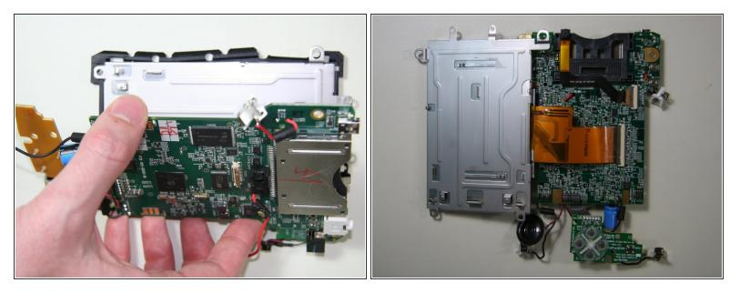
• Carefully flip the motherboard over by pivoting away from the screen assembly along the long edge with the microphone and speaker, as shown.
