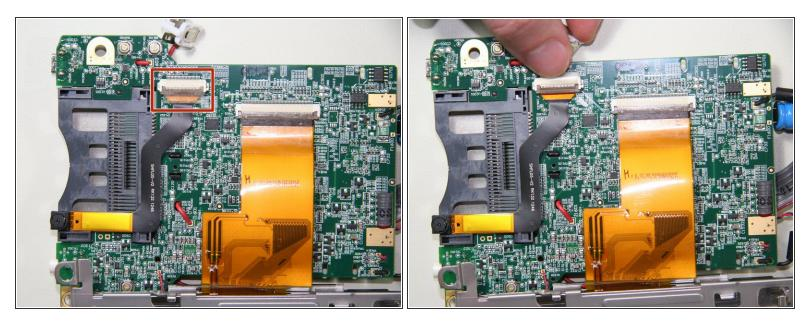
Peel back the tape on the camera ribbon cable connector.
