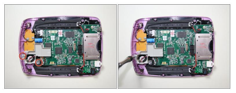
• Use a Phillips #1 screwdriver to remove two 5.5mm screws from the plastic speaker holder.
