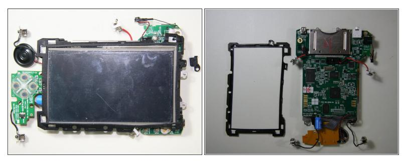
(i) The rubber screen border may separate on its own after removing the front cover from the screen assembly and motherboard. Set it aside if it comes off.
