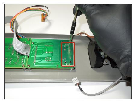
These are the 12 contacts that must be de-soldered in order to remove the data entry slide bar, 4 are electrical and 8 secure the housing.
