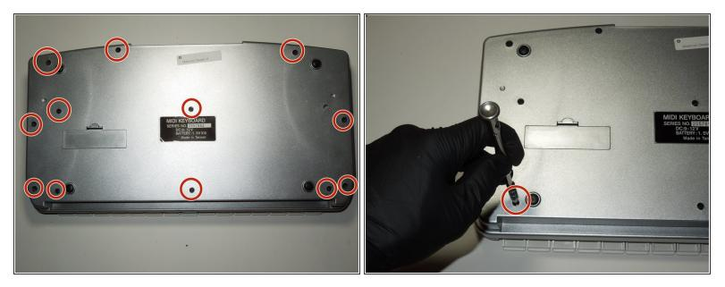
• Remove the 8 mm M3 Phillips head self tapping machine screws.
