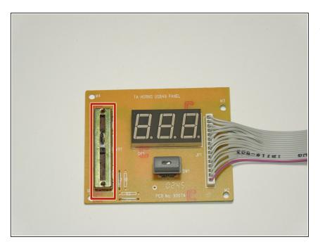
• After de-soldering the part, you will be able to remove it and replace it.
