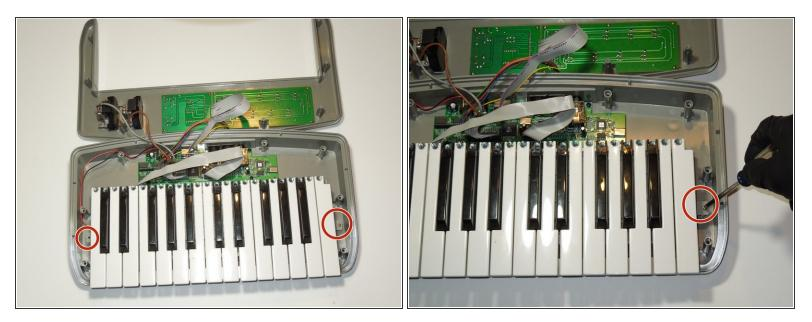
Remove the two highlighted 10 mm M3 galvanized machine screws using the J1 head fro the iFixit Tool Kit or a comparable tool.
