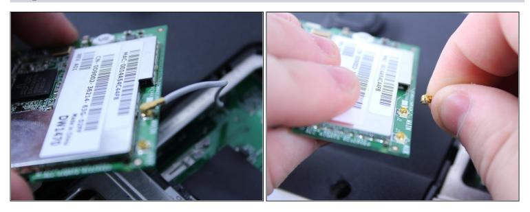
• To remove the wire, hold the wireless chip firmly and pull the connection straight up off of the chip.
