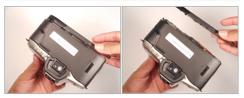
(i) Once all the screws are removed, the panel should easily come off.
