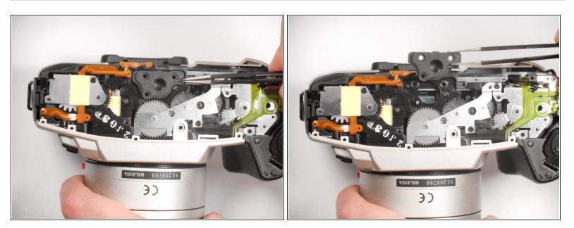
Use the tweezers to gently remove the tripod socket, and replace it.
