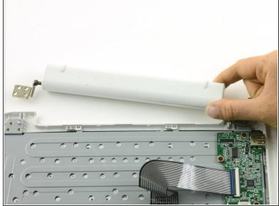
Lift the hinge away from the device.
