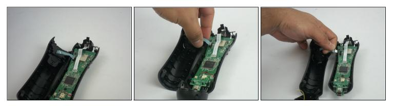
• Remove the blue strip that is connected to the trigger button from the motherboard.
