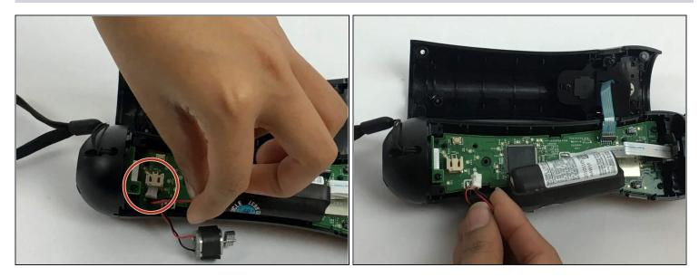
• Gently pull on the white piece connecting the battery and the connector.
