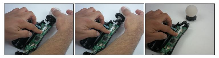
• Cautiously remove the circular white piece at the top without removing the LED inside.
