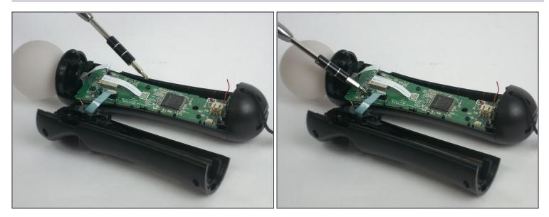
• Remove the two 1.2mm Phillips #1 screws.
