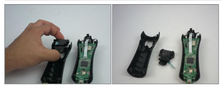
• Remove the trigger button from the controller.
