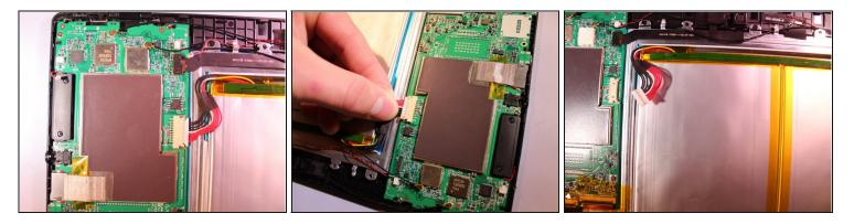
• Using tweezers, remove the electrical connector that connects to the battery to remove the power to the battery.
