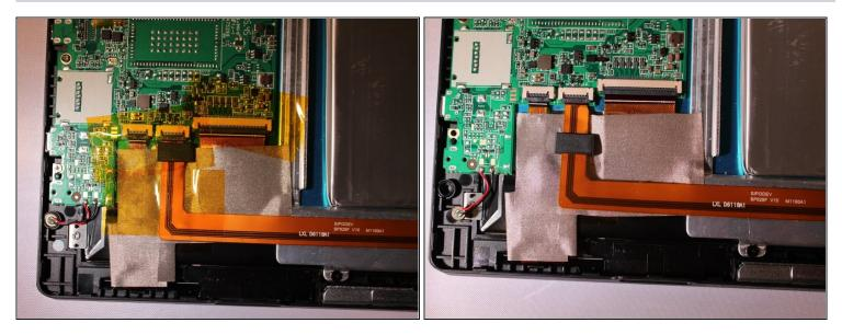
• Peel the yellow tape off from on top of the electrical connectors.
