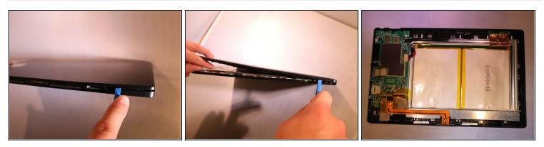
• Using a plastic tool and the <u>plastic card</u>, gently pry off the back cover.
