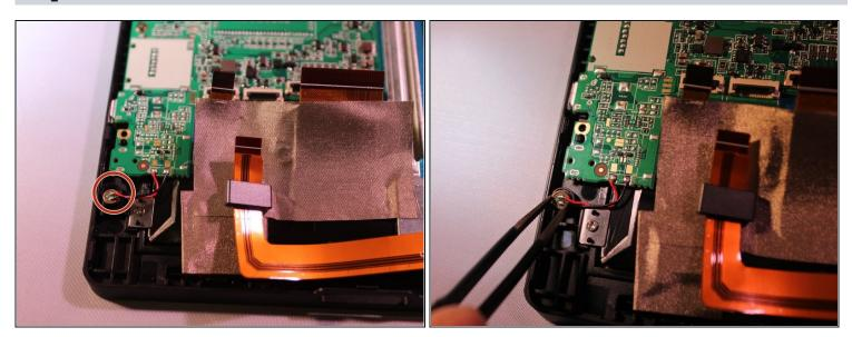
Using tweezers, remove the microphone from the the plastic cover.
