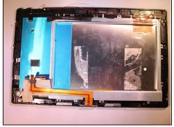
• Remove battery by prying off with card.
