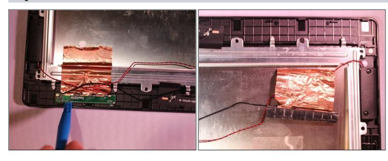
• Peel back the copper color electrical connector with blue opening tool.
