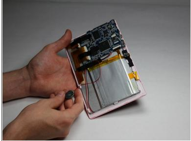
• Using the spudger tool, detach the speaker from the back of the screen.
