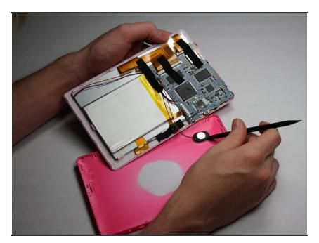
Using your spudger tool, remove speaker from the backboard.
