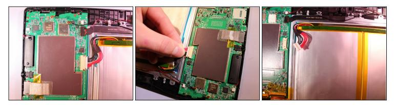
• Using <u>tweezers</u>, remove the electrical connector that connects to the battery to remove the power to the battery.
