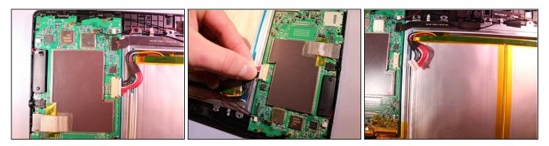
• Using tweezers, remove the electrical connector that connects to the battery to remove the power to the battery.
