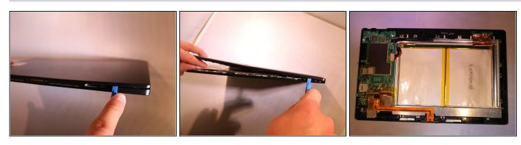
• Using a plastic tool and the <u>plastic card</u>, gently pry off the back cover.
