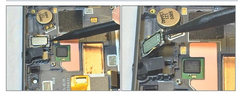
• Use the pointy end of the spudger to firmly lift the earpiece speaker out of the socket.
