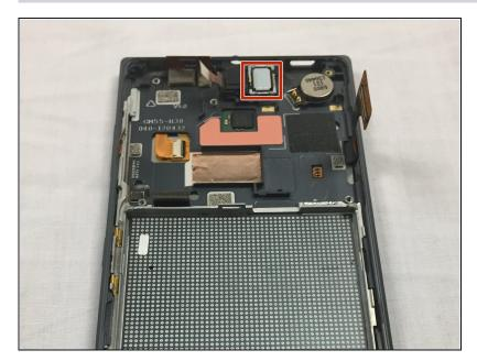
The speaker is located at the top of the device to the right of the headphone jack.
