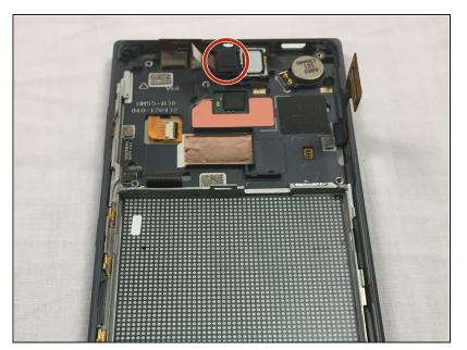
The headphone jack is located at the top of the phone. It is flush up against a circular hole in the frame of the device.
