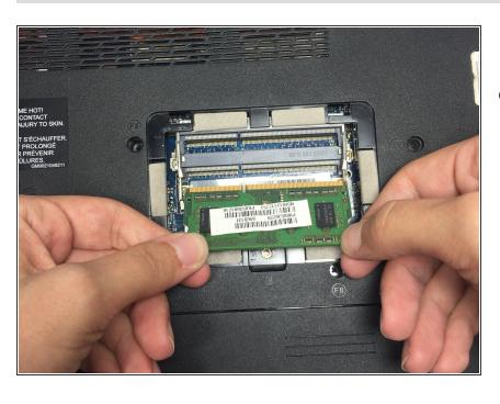
Remove the lower RAM chip from its socket by gently gripping the left and right edges with your fingers and pulling the chip towards your body until it slides completely free of the computer. To reassemble your device, follow these instructions in reverse order.
