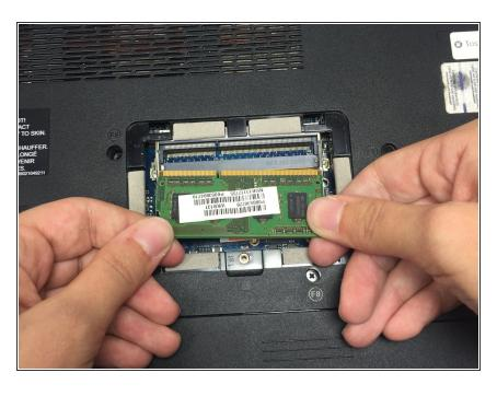
Remove the upper RAM chip from its socket by gently gripping the left and right edges with your fingers and pulling the chip towards your body until it slides completely free of the computer.
