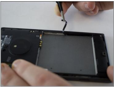
Remove the black strips on both sides of the battery compartment.
