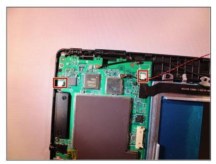
Remove 2 electrical connectors that connects to the speaker using flat tweezers.
