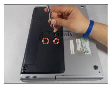
Unscrew the two 2x5mm screws with a #00 Phillips screwdriver.
