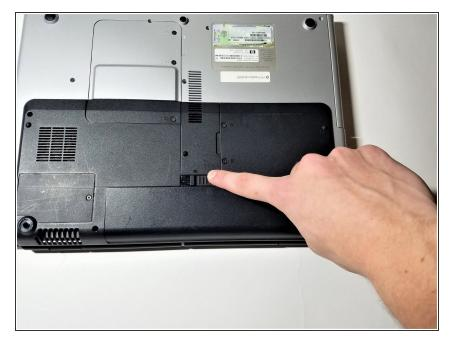
Slide the battery release latch to the right and hold in place.
