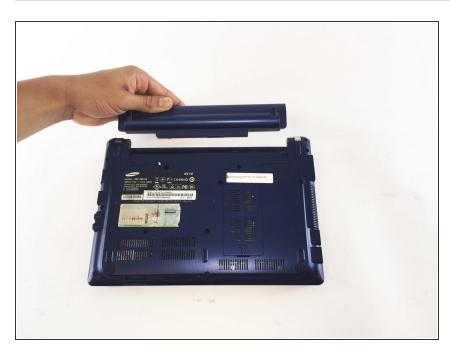
Pull the battery up from the device.
