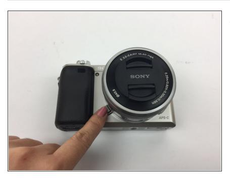
Press and hold the release button next to the lens on the front of the camera.
