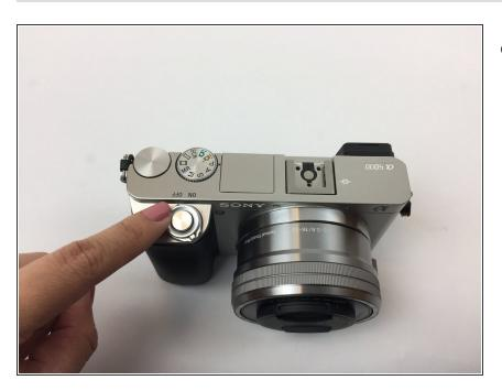
Make sure the camera is turned off by turning the switch to OFF.
