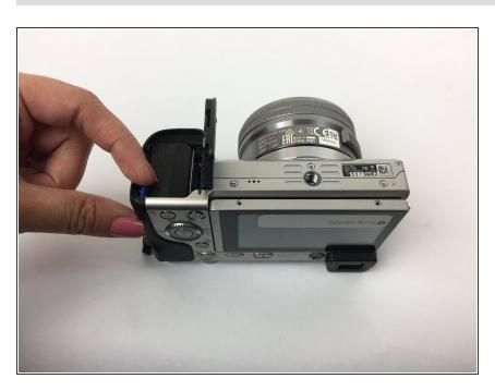
Push the latch back to release battery.
