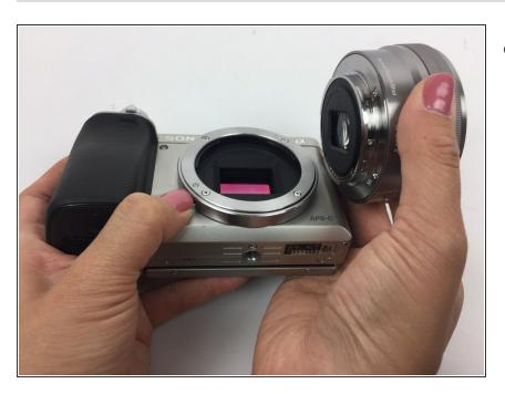
While holding the release button, twist the lens counterclockwise and pull it off.
