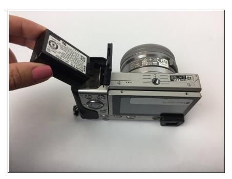
The battery can now be taken out of its compartment.
