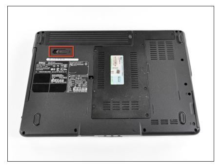
Locate the battery release switch on the bottom of the laptop.
