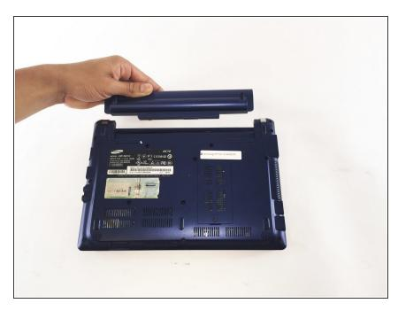
Pull the battery up from the device.
