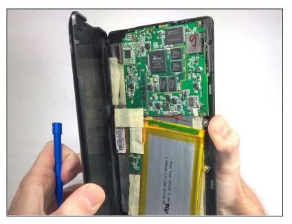
Pull the cover off of the device once about three quarters of the cover has been pried open using the plastic opening tool.
