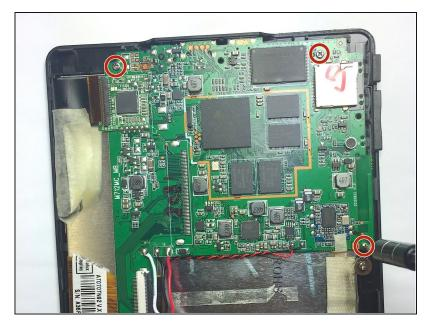
Use the nut driver and J00 bit to remove the three 4 mm screws.
