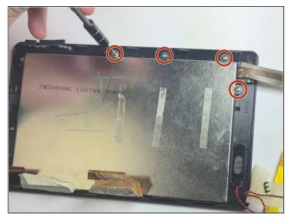
Use the nut driver and the J0 bit to unscrew the four 4 mm screws
