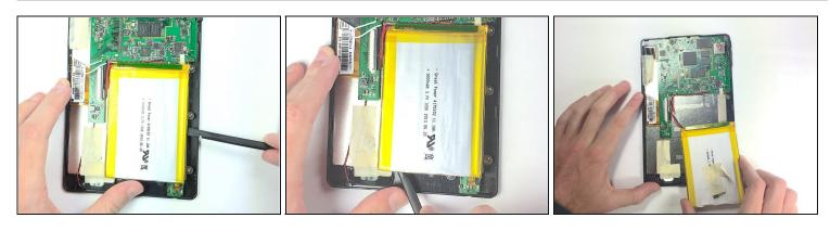
• Pry the battery from the base using the nylon spudger and move it away from the motherboard.
