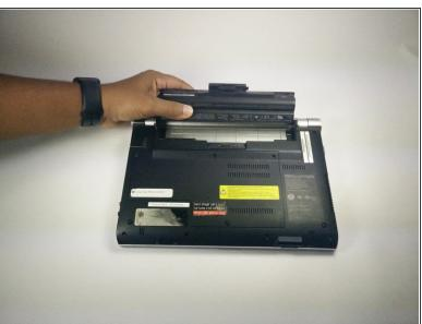
While still holding the "Slide" latch, lift battery up and out of the device.
