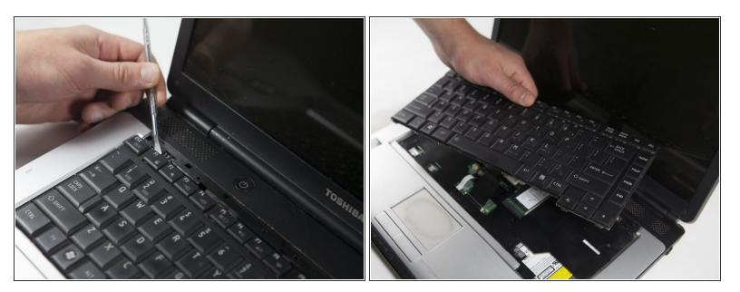
Use the metal spludger to push the keyboard in the direction of the track pad and then lift the keyboard up.
