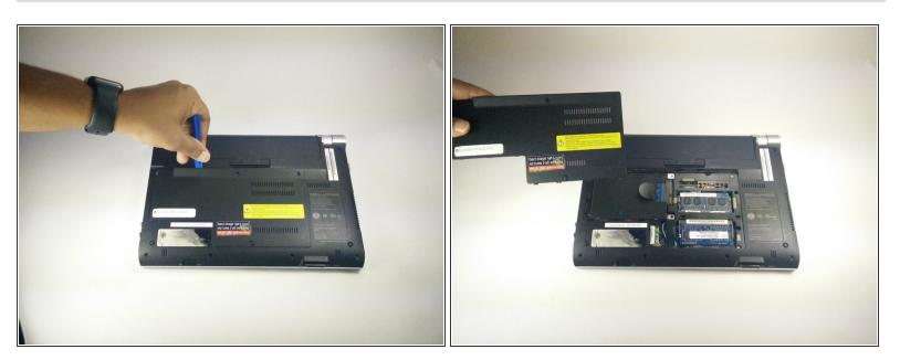
• Use a plastic opening tool to pull up on the plate and remove from device.
