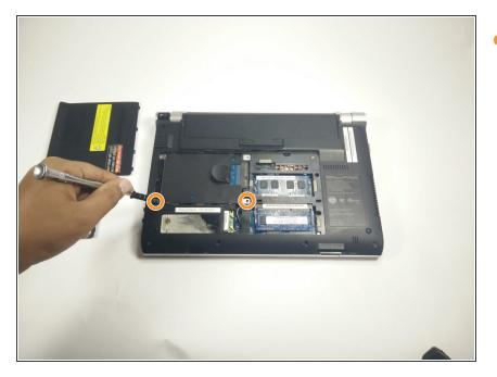
Locate screws holding in the hard drive and remove.
