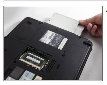
Fully remove the drive by pulling it all the way out of its socket.
