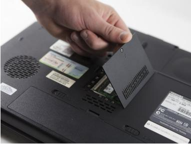
• Remove the panel that houses the RAM chips by removing the screw that secures it into its spot.
