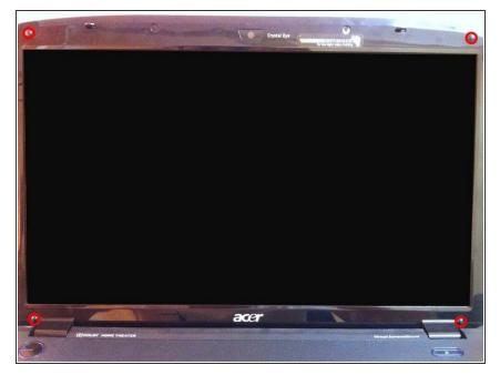
Remove the 4 rubber supports from the screen. Then remove the screws underneath.
