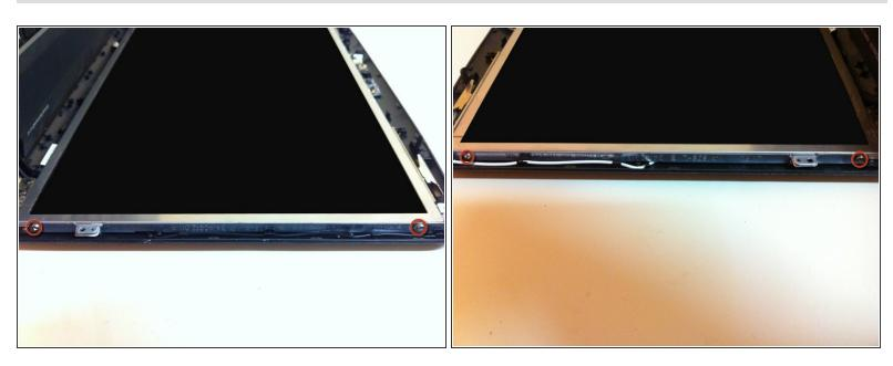
• Remove the 4 screws in the side of the LCD. Screen should be able to come of the frame
