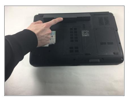
Lift the battery up, and it should just come right off. You should see the label with the part number.
