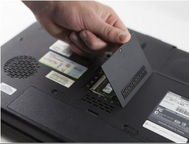
• Remove the panel that houses the RAM chips by removing the screw that secures it into its spot.
