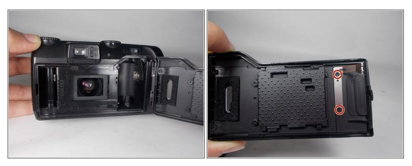
Once the compartment is open and unscrew the two 0.5mm Phillips screws that hold the spring in place. Replace the spring with a new one.
