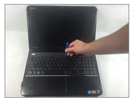
• Slide a plastic opening tool into the slots on the top of the keyboard.
