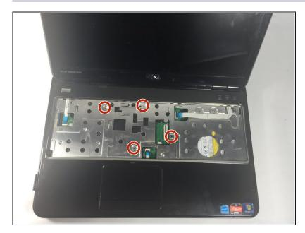
• Turn the computer over and open the display as far as possible and remove the four 5 mm Phillips # 0 screw holding the palmrest in place.
