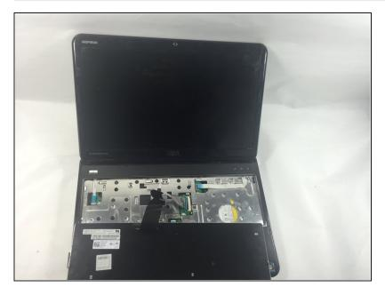
• Flip the keyboard over and place it on the front of the device making sure not to pull out the keyboard cable.
