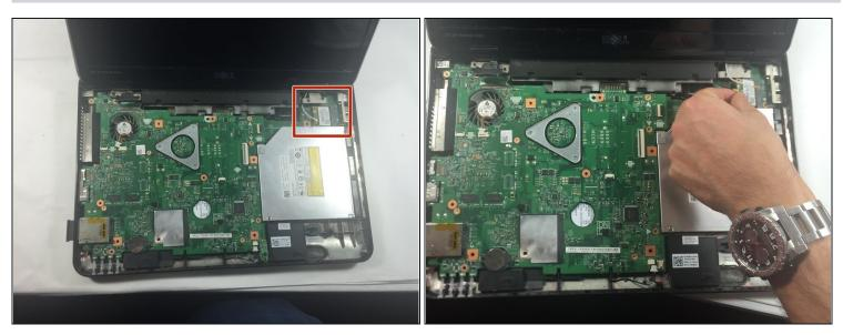
• Disconnect the black and white antenna cables from the Mini Card.
