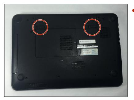
Slide both of the battery release latches on the bottom of the device in towards the center of the computer.
