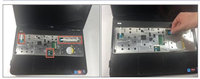
• Disconnect the power button board cable, touch pad cable and the hot key board cable from the connectors.
