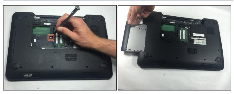
• Insert a small screwdriver into the hole and slide the optical drive away from the center of the device. This will slide the optical assembly out from the side of the device.
