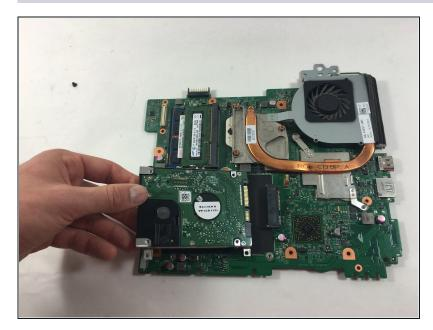
• Pull gently on the end of the hard drive that is farthest away from the fan, it will come out easily.
