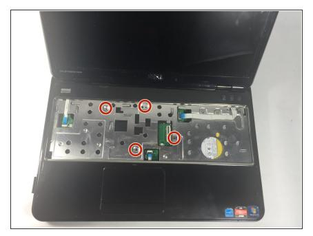
Turn the computer over and open the display as far as possible and remove the four 5 mm Phillips # 0 screw holding the palmrest in place.
