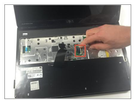
Lift up the connector latch and remove the keyboard cable. The keyboard is now free from the device.
