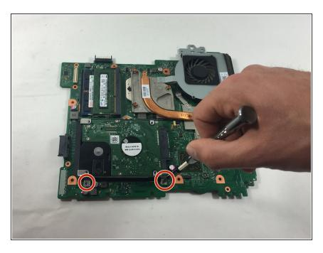
Remove the two 5 mm Phillips # 0 screws holding in place the hard drive.
