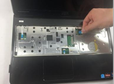
Disconnect the power button board cable, touch pad cable and the hot key board cable from the connectors.
