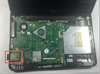
Remove the SD card by pressing the SD card slot, on the side of the device, inside the device until
