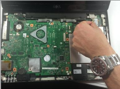
• Disconnect the black and white antenna cables from the Mini Card.
