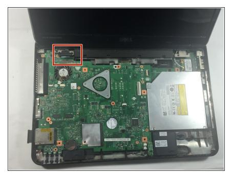
Unplug the rectangular black LCD cable attached to the system board towards the upper left hand corner.
