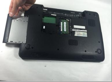
Insert a small screwdriver into the hole and slide the optical drive away from the center of the device. This will slide the optical assembly out from the side of the device.
