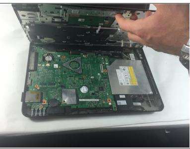
Use a plastic opening tool to carefully pry out the palmrest assembly and lift it off the computer base.
