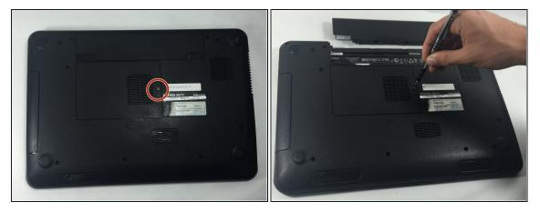
• Remove the 5 mm Phillips # 0 screw in the middle of the device.
