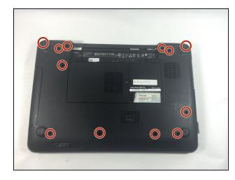
• Turn the computer over and remove the twelve 5 mm Phillips # 0 screws on the back of the device.
