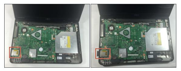
• Remove the SD card by pressing the SD card slot, on the side of the device, inside the device until you hear a click. Then release your pressure on the slot then gently slide the SD card out.
