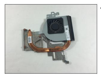
• Lift the fan compartment up to remove it from the systemboard.
