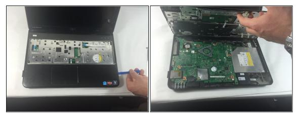
• Use a plastic opening tool to carefully pry out the palmrest assembly and lift it off the computer base.
