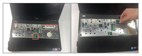
• Disconnect the power button board cable, touch pad cable and the hot key board cable from the connectors.
