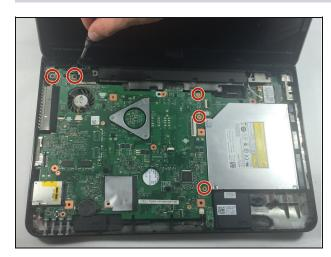
Unscrew the five 5 mm Phillips # 0 screws located in the red circles, found on the system board.
