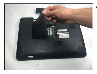
• Remove the module cover pressing in the release tabs and pulling the cover up and away from the base of the device.
