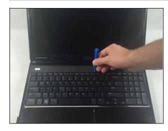
• Slide a plastic opening tool into the slots on the top of the keyboard.
