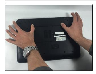
• Slide and lift the battery up and out from the device.
