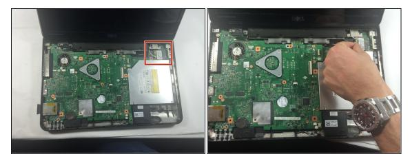
• Disconnect the black and white antenna cables from the Mini Card.
