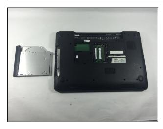
• Slide the optical drive assembly the rest of the way out of the device.
