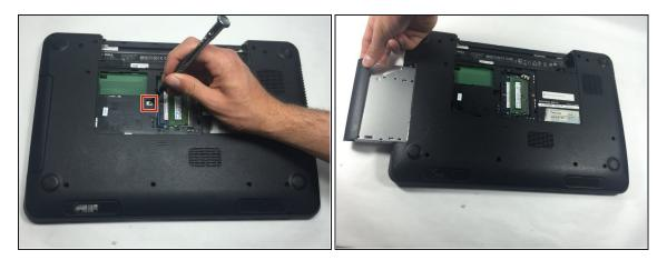
• Insert a small screwdriver into the hole and slide the optical drive away from the center of the device. This will slide the optical assembly out from the side of the device.
