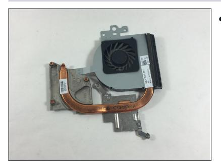
• Lift the fan compartment up to remove it from the systemboard.
