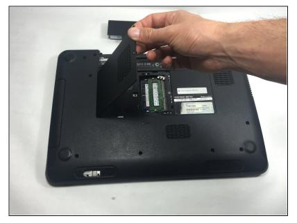
• Remove the module cover pressing in the release tabs and pulling the cover up and away from the base of the device.
