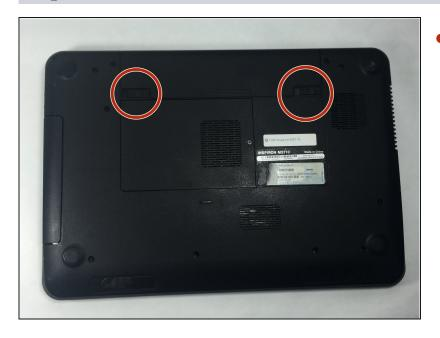
Slide both of the battery release latches on the bottom of the device in towards the center of the computer.
