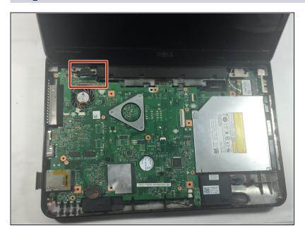
• Unplug the rectangular black LCD cable attached to the main board towards the upper left hand corner.
