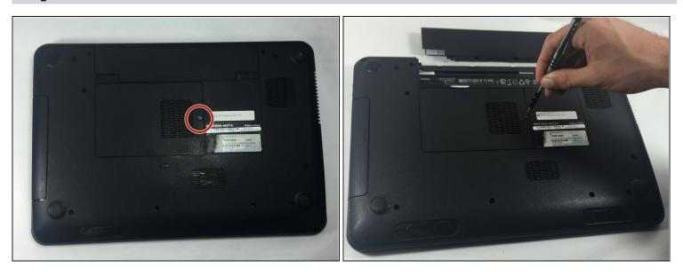
• Remove the 5 mm Phillips # 0 screw in the middle of the device.
