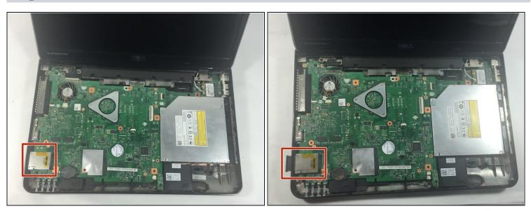
• Remove the SD card by pressing the SD card slot, on the side of the device, inside the device until you hear a click. Then release your pressure on the slot then gently slide the SD card out.
