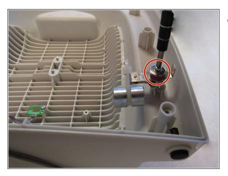
Unscrew the Phillips #2 10 mm screw from the safety weight on the rear housing panel.
