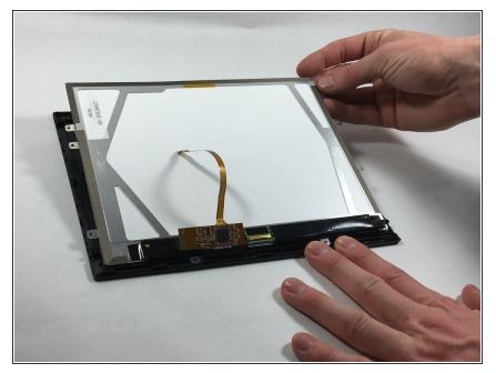
• Lift and carefully remove the LCD display from the front cover.
