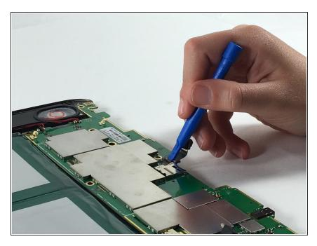
• Use the plastic opening tool to lift the connector up and remove the camera.
