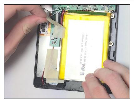
Remove masking tape from the battery.
