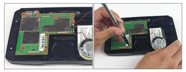
• Using a T5 Torx screwdriver remove the eight screws attaching the motherboard to the case
