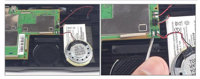
• Grasp the wire connecting the motherboard and pull the wares connecting it.
