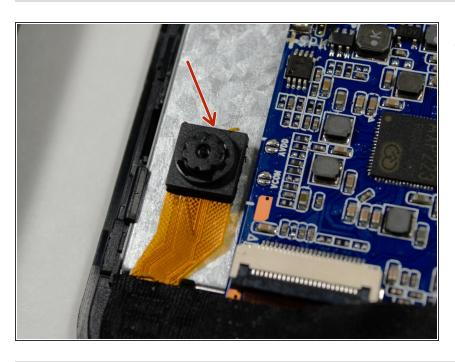
Gently dislodge the camera using the Metal Spudger. The camera is now ready to be replaced.
