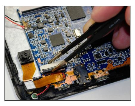
Use a pair of Precision Tweezers to squeeze the clip of the ribbon wire to release it.
