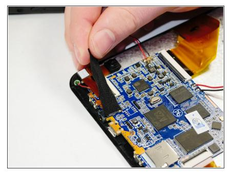
Carefully remove the black electrical tape connecting the motherboard to the ribbon wire.
